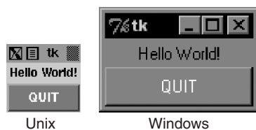
Figure 19–3 Tkinter Label and Button widgets (tkhello3.py)
